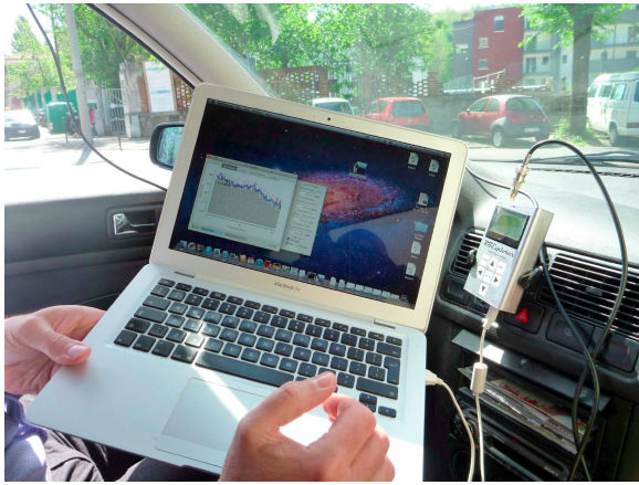
Fig. 4. Laptop and RF Explorer inside the car during a measurement.
