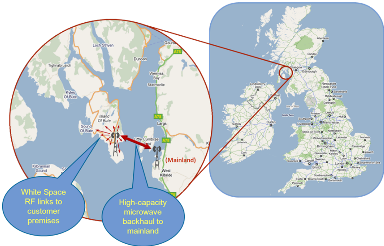
Figure 9.1: High-level illustration of trial white space network on Bute.
