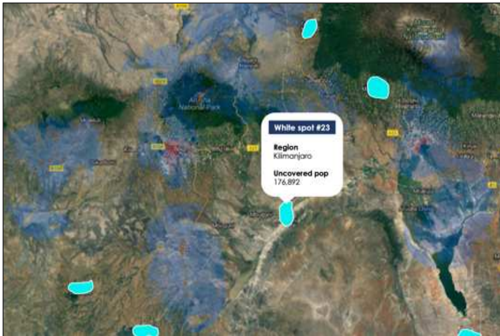
Figure A1.2. Masae Analytics algorithm with granular population density open data and coverage information to detect the most promising zones (“white spots”) for the installation of new base stations
